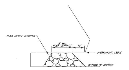
NOTE: BACKFILL FULL LENGTH OF OVERHANGING LEDGE
