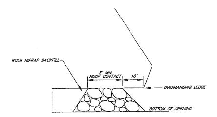
NOTE: BACKFILL FULL LENGTH OF OVERHANGING LEDGE
