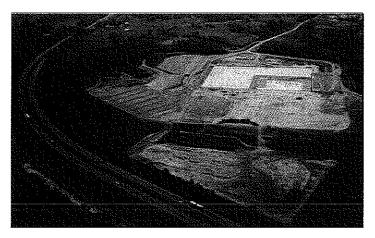
Aerial view of facility in late summer. The 8.5-acre distribution center under construction is located in the upper right corner with parking areas to the left. A 7.5-acre wetland mitigation area was designed and constructed between Interstate 77 and the new facility. Future expansion area was also brought up to grade allowing Coldwater Creek to potentially double their building size with minimal earthwork activities.
