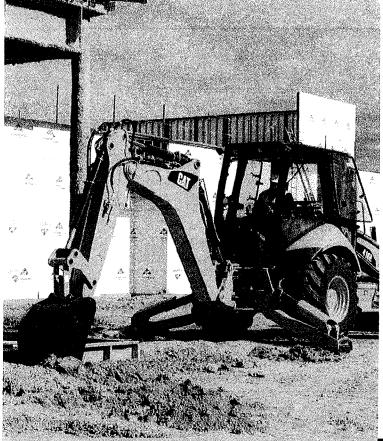
The 416E has a load-sensing, closed center hydraulic system, which closely matches power and flow to the demand needed by the implements. So whether you're in full trenching mode, or delicately digging around services, you are in control. In applications such as production trenching, speed is important and the system will match the flow needed to get the job done quickly and efficiently. The load-sensing hydraulic system also delivers:
