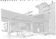
This office complex is being designing using BIM software (Revit). Starting with the existing structure, the team used Revit and other 3-D modeling tools to assist the client and user in visualizing the design. As the technical documents are developed, Revit is being used to allow for more accurate coordination among the disciplines. LAI's team is further utilizing BIM to accelerate the design schedule.
