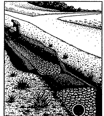
Wrapping a subsurface drainage system with a Geotex® nonwoven geotextile will improve roadway life.
