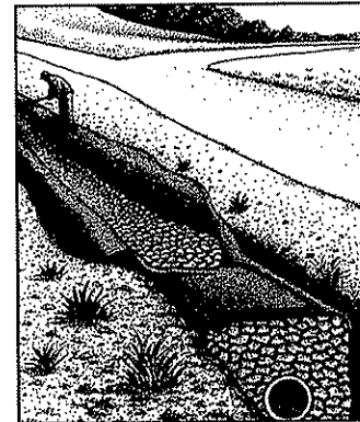
Wrapping a subsurface drainage system with a Geotex® nonwoven geotextile will improve roadway life.
