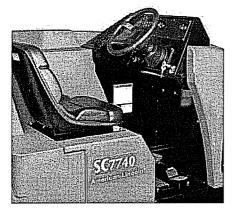
A tilt steering wheel and reliable rocker switches make the controls in the operator's compartment easy to use.
