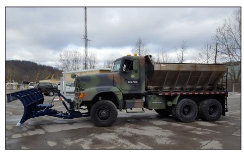
The six tractor trailers purchased by the Division of Highways were converted into snowplows and salt spreaders. These vehicles will be used along Corridor H, which runs between the Grant and Tucker county lines and often receives large amounts of snow. Due to the mountainous and winding roads in this area, it is critical to have the proper vehicles to treat the roads during dangerous winter weather.
