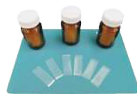
Standard Samples Containing Phthalate Ester for Py-GC/MS
