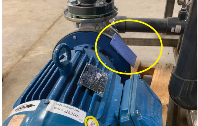
EZ Brine Pump: Located on the top and side of the pump.
