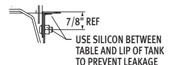
Sectional View Showing Table Connections
