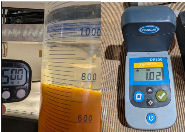
Appendix 4: After 5 minutes of settling, the 0.75 ppm dose settled 600 mL more than the 0.25 ppm dose and the total iron after 5 minutes was 1.02 mg/L at the 0.75 ppm dose compared to 3.08 mg/L at the 0.25 ppm dose.
