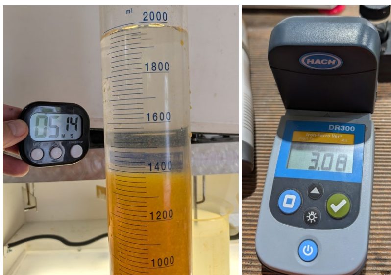
Appendix 2: After 5 minutes significant settling occurred and a sample of the top of the supernate showed a total iron concentration of 3.08 mg/L. Some floc are visible near the solid/liquid interface.
