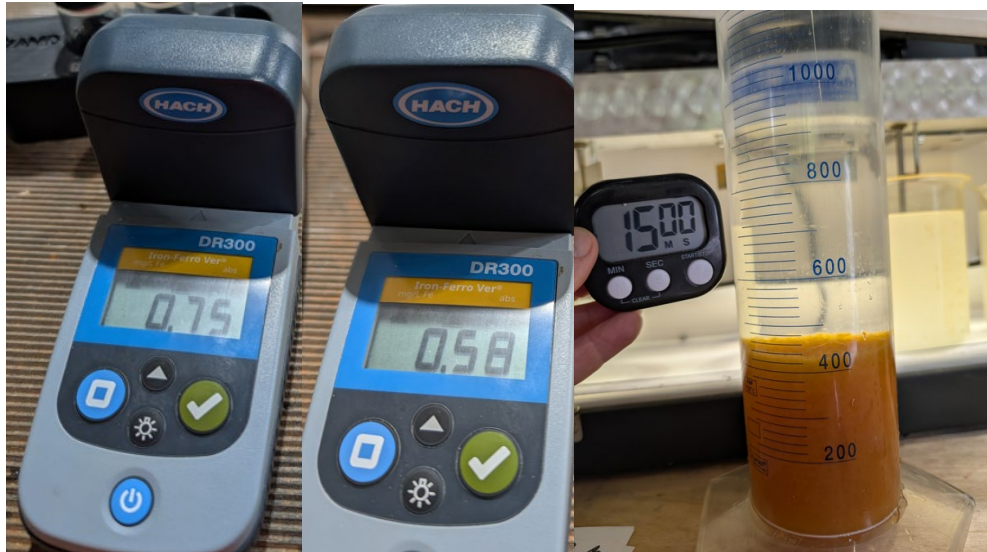
Appendix 9: After 9 minutes of settling the total iron in the supernate was 0.75 mg/L and after 15 minutes the total iron was 0.58 mg/L.
