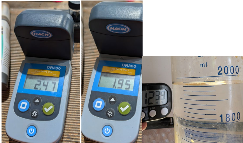
Appendix 3: After 9 minutes of settling the total iron in the supernate was 2.47 mg/L and after 15 minutes was 1.95 mg/L. After 12 minutes of settling time the supernate is visibly clear.
