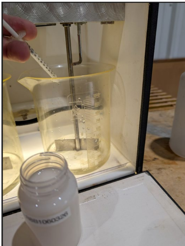
Figure 2: Dosing 1 mL of emulsion polymer into 100 mL of water (1% solution by wt.) to “invert” the polymer and prepare to make a dilute polymer solution for dosing.
