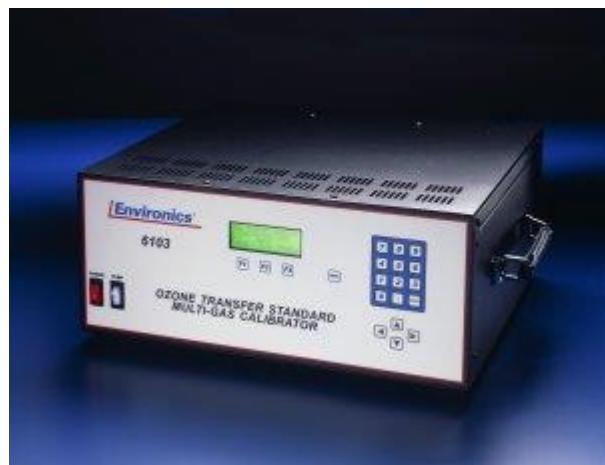
The internal photometer measures the actual amount of ozone generated, and corrects for errors, using closed-loop PID control. The photometer also allows an external source of ozone to be analyzed and displayed on the screen. The external ozone connector to a separate sample port, allowing for simultaneous gas blending while monitoring the external ozone source.
