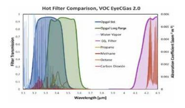
The EyeCGas Multi camera features replaceable filters that enhance its flexibility and performance for detecting various gases. The camera comes with three key filters: a Standard VOC filter, a Heavy alkanes & longrange VOC detection filter, and a CO<sub>2</sub> filter. These filters allow users to monitor a broad spectrum of gases with a single device, making the camera highly adaptable across different industrial applications. Operators can easily switch between filters depending on the target
