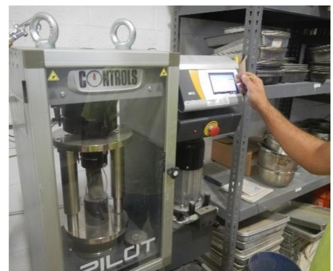
Photo shows Stahl Sheaffer’s Rock Comprehensive Strength Test, completed for this project in-house at our soils & Materials Lab.
