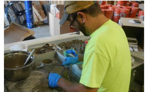
Photo demonstrates Stahl Sheaffer’s FDR with proctor tests completed for the project at Stahl Sheaffer’s Soils & Materials Lab.
