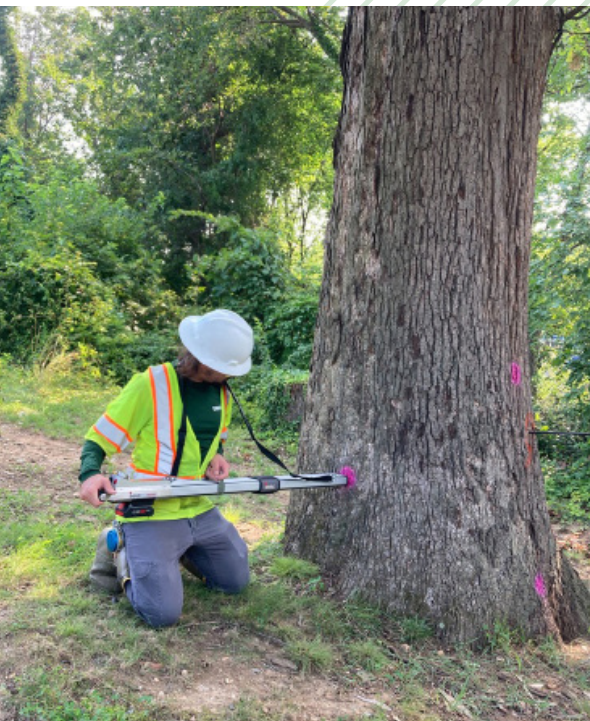
WSSI arborist using a resistance drill to detect decay in a white oak.
