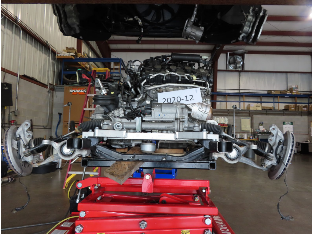
ENGINE/TRANSMISSION REMOVAL AND REPLACEMENT (8.00 LABOR HOURS)
