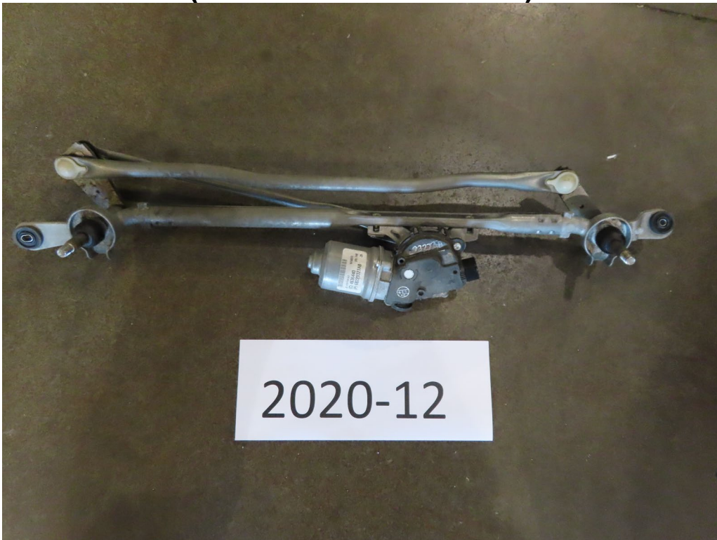
WIPER MOTOR REMOVAL AND REPLACEMENT (0.33 LABOR HOURS)
