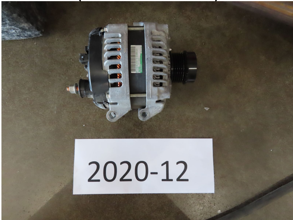
ALTERNATOR REMOVAL AND REPLACEMENT (3.50 LABOR HOURS)
