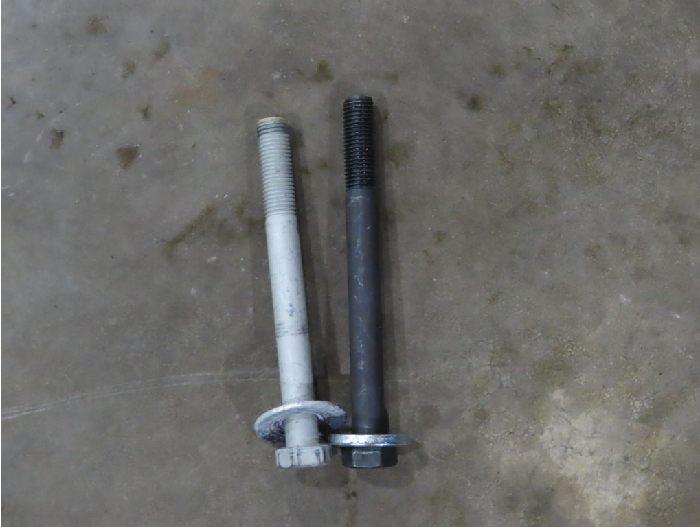
REPLACED FRONT SUBFRAME BOLTS AND WASHERS (3,445 TEST MILES)
