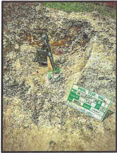
Image 7.2: Post Plug sampling after cutoff
