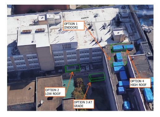
The MEP needs for the existing 12-table gross anatomy lab were evaluated. The lab was approximately 30 years old and in need of updated HVAC systems, as well as improved redundancy of systems. Existing lab and systems were located with difficult access. The study examined multiple solutions regarding first cost, maintenance, and level of operation. Code ramifications and expanded use of the lab were considered. Design criteria were suggested to optimize construction and operation costs.
