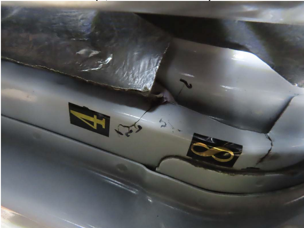
CRACKS ON BACKSIDE OF CURBSIDE FRONT WHEEL WELL INNER FENDER ABOVE FRAME RAIL (7,517 TEST MILES)
