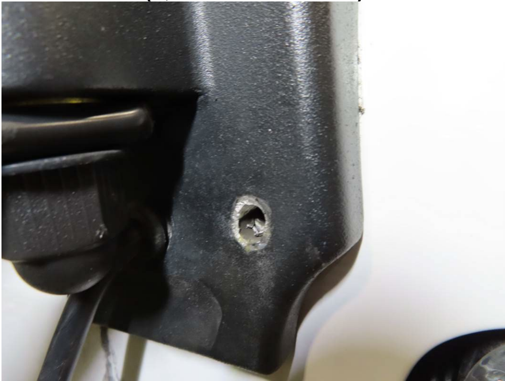
BROKEN MOUNTING SCREW ON CURBSIDE FENDER MIRROR (5,598 TEST MILES)
