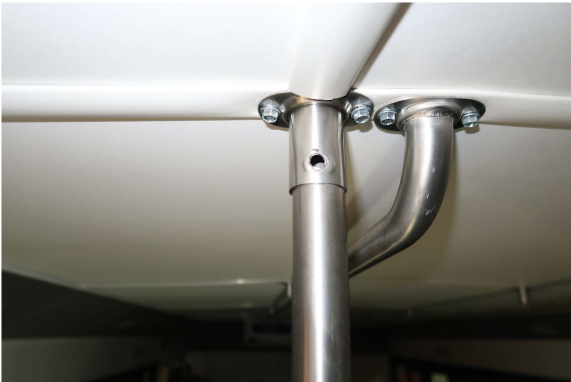
BOLT MISSING AT TOP OF GRAB BAR AT PASSENGER ENTRANCE (2,037 TEST MILES)
