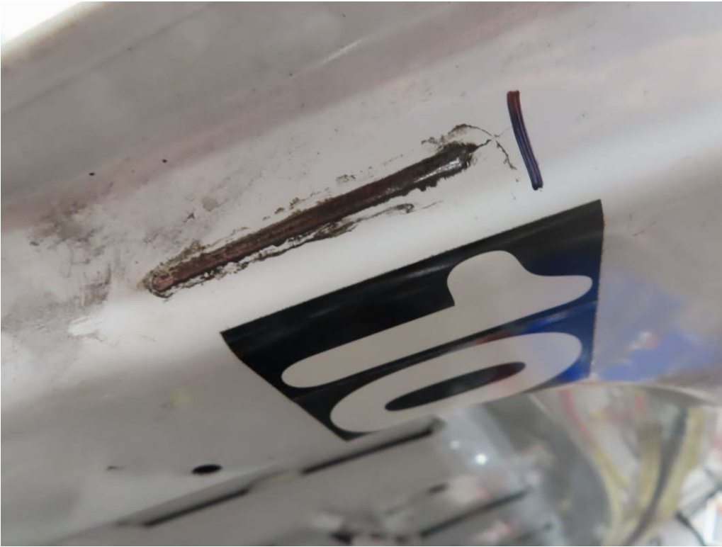
CRACK ON HOOD WHERE MIRROR BRACKET IS HITTING (7,517 TEST MILES)
