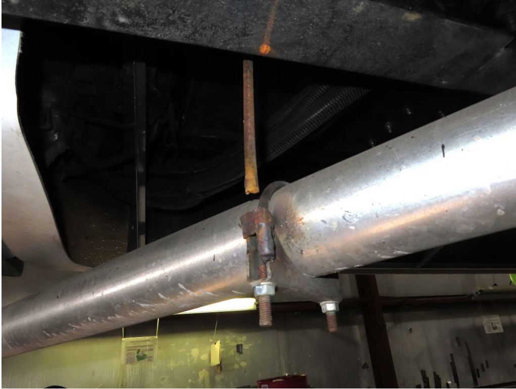
BROKEN EXHAUST HANGER BRACKET (972 TEST MILES)
