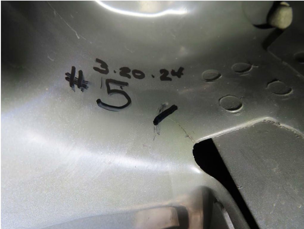
CRACK ON UNDERSIDE OF BODY UNDER REAR BOLT ON DRIVER'S SEAT (5,598 TEST MILES)
