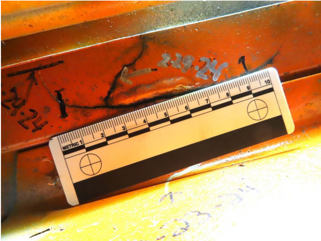
CRACK ON UNDERSIDE OF BODY WHERE RIVETS WERE INSTALLED (4,561 TEST MILES)
