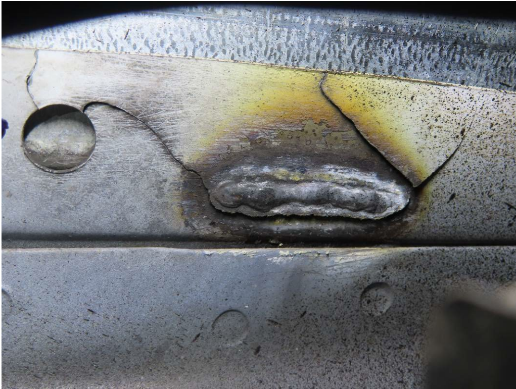
CRACKS ON FORD BODY WHERE IT ATTACHES TO BUS BODY (4,561 TEST MILES)
