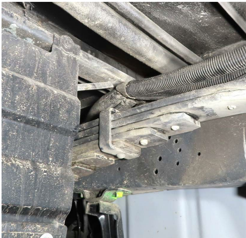
STREETSIDE REAR LEAF SPRING HITTING COOLANT LINES AND WIRES (3,409 TEST MILES)
