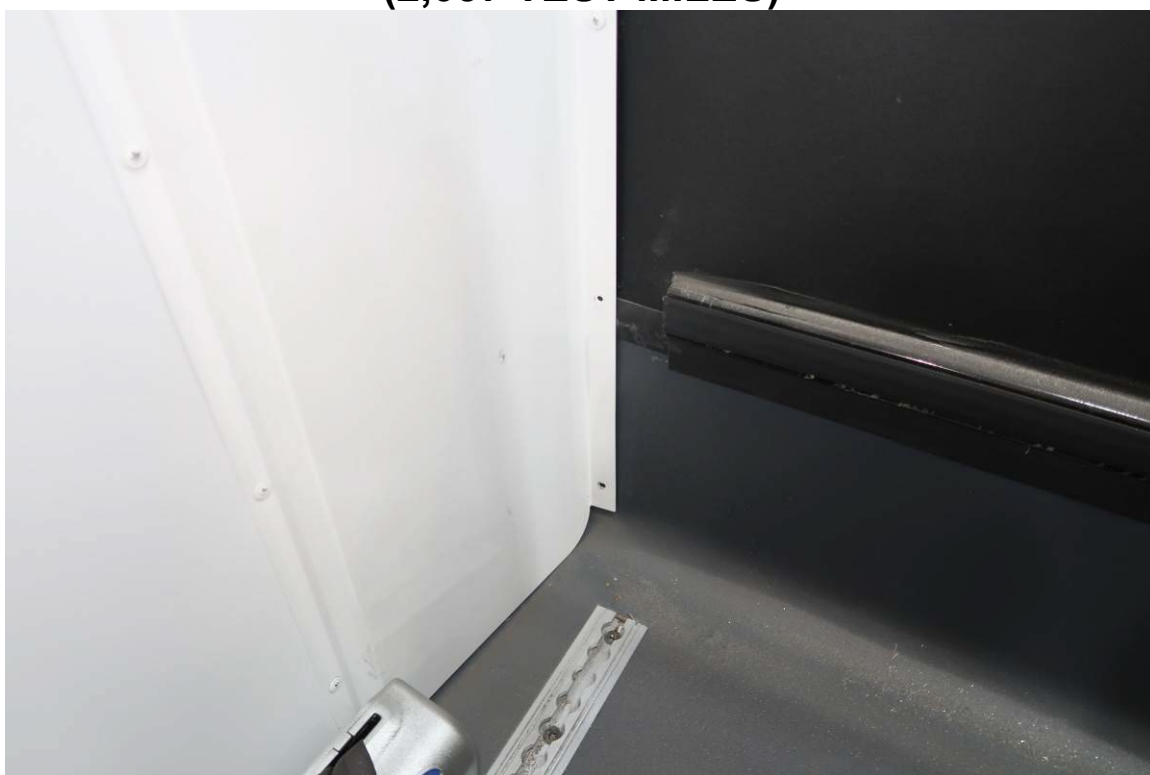
SCREWS MISSING BY REAR EXIT DOOR (2,037 TEST MILES)
