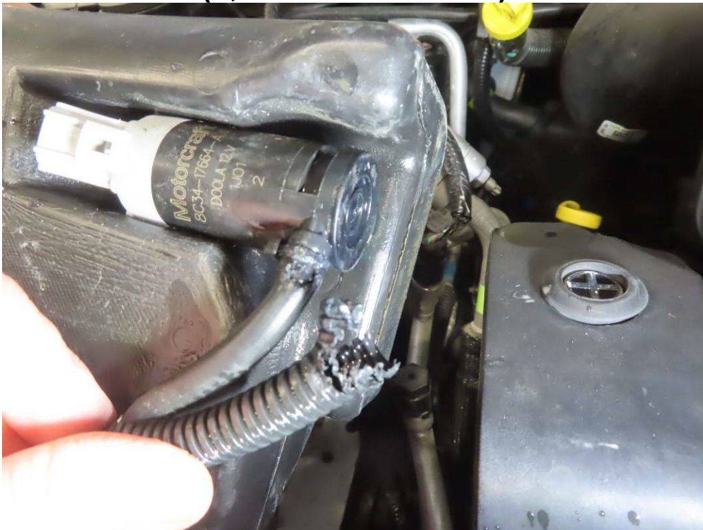
WINDSHIELD WASHER TANK HOSE WORN THROUGH (6,863 TEST MILES)
