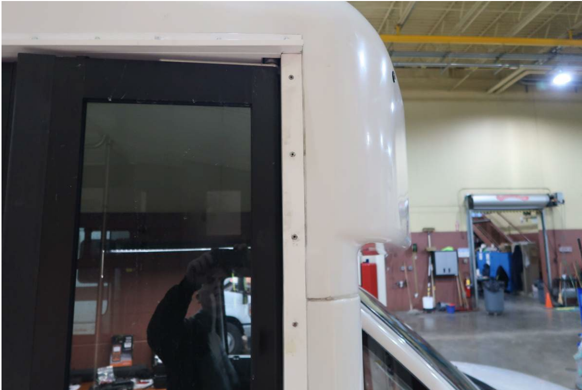
STEEL RIVETS INSTALLED IN MAIN PASSENGER ENTRANCE DOOR SURROUND (2,037 TEST MILES)
