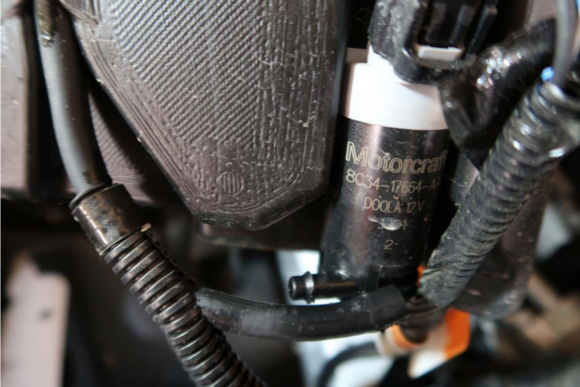
HOSE CAME OFF OF WINDSHIELD WASHER FLUID PUMP (233 TEST MILES)
