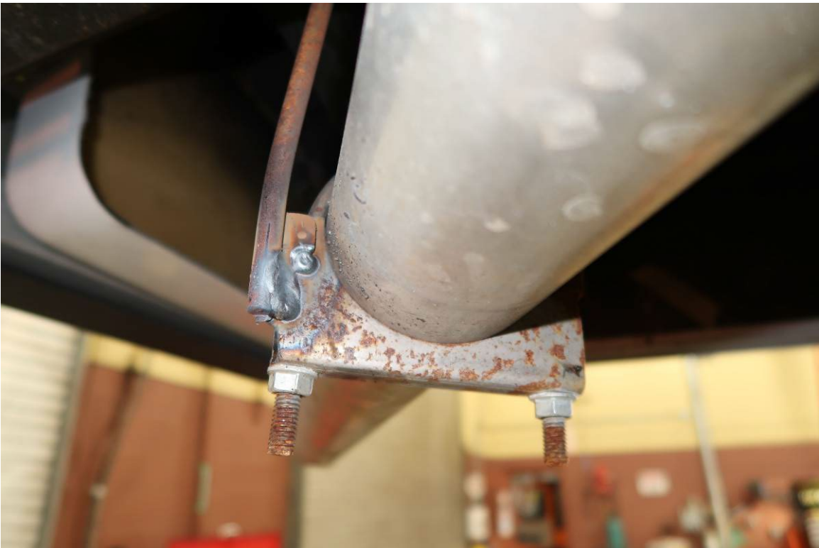
EXHAUST HANGER WELDED BACK INTO PLACE (233 TEST MILES)
