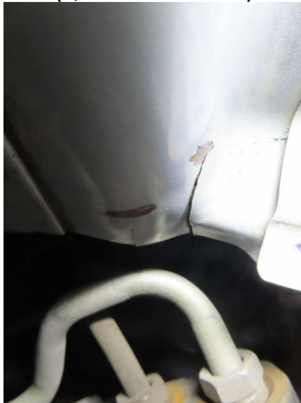
CRACKS ON STREETSIDE FORWARD PART OF INNER FENDER ABOVE FRAME FORWARD OF COIL SPRING (7,517 TEST MILES)
