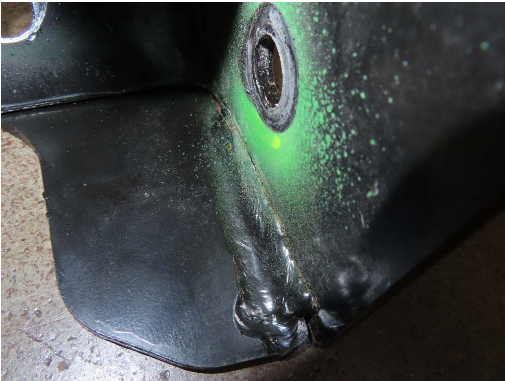
CRACKED WELD ON STREETSIDE MOTOR MOUNT (4,561 TEST MILES)
