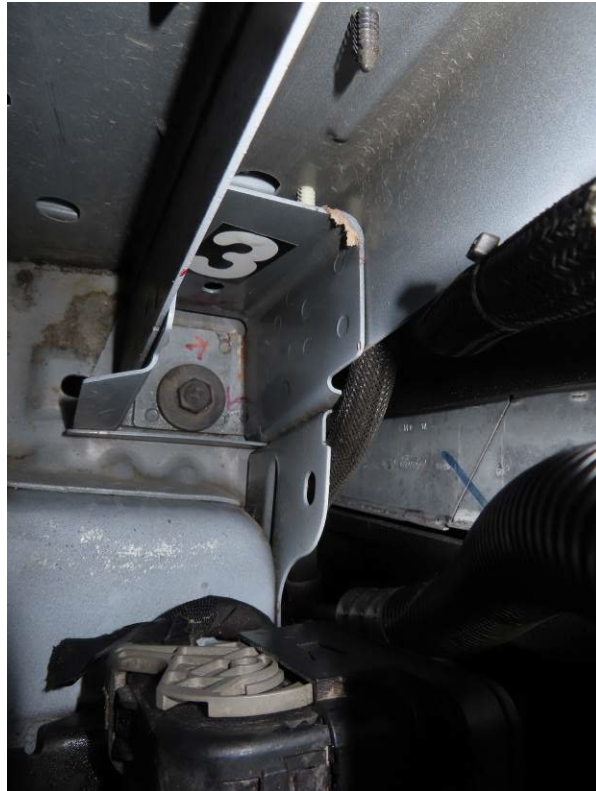
CRACK ON CORE SUPPORT ON STREETSIDE (5,598 TEST MILES)
