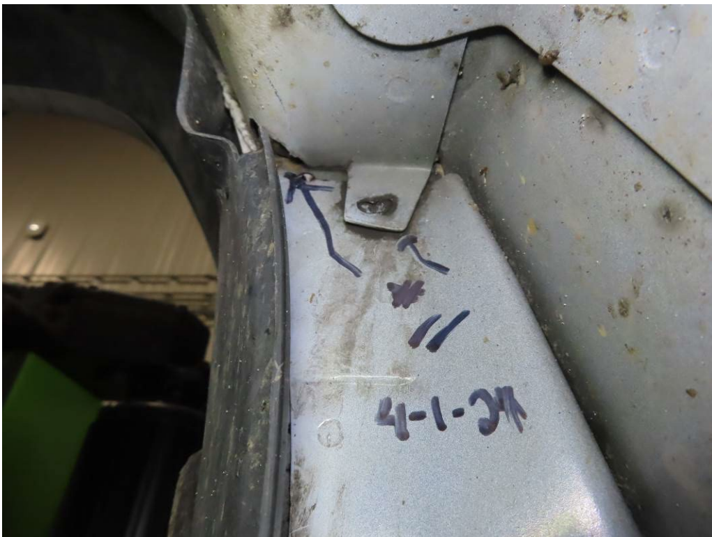
PIECE MISSING AND CRACK ON CURBSIDE INNER FENDER (7,517 TEST MILES)
