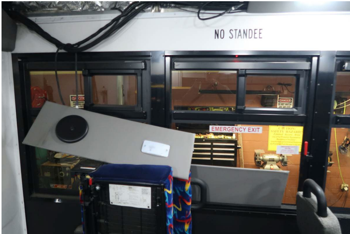
PANELS ABOVE PASSENGER SEATS FELL (6,256 TEST MILES)
