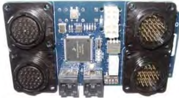
Figure 5. Typical CAN circuit board – simple, rugged, reliable
