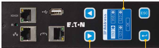
Local buttons allow for easy menu navigation and simplify setup
