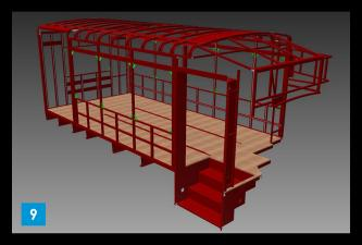
Plywood flooring is secured with an adhesive to eliminate squeaks and movement.
