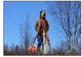
field information. Total station instruments equipped with data collectors are utilized for complete field to office automation allowing for high levels of productivity in the field. The latest versions of software are then used to process survey data and create drawings or required end products.
