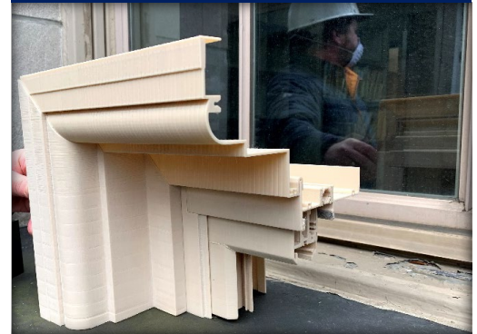
3D-printed window prototype used to verify complex historic window replica profiles
