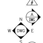
ELEVATION VIEW REFERENCE TAG INTERIOR ELEVATION
