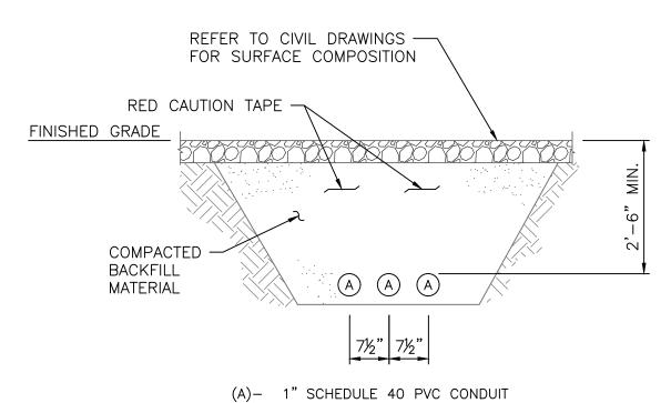
THREE-CONDUIT UNDERGROUND ELECTRICAL CONDUIT DUCT BANK 3E501 SCALE: N.T.S.
