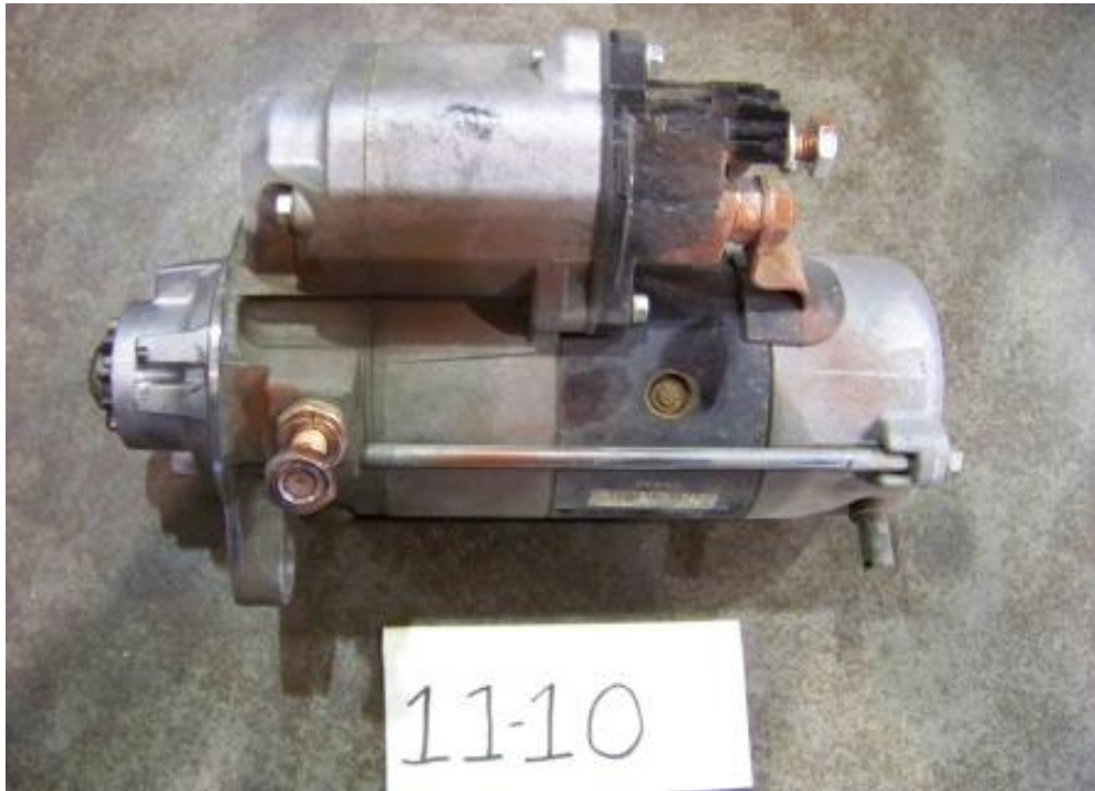
STARTER REMOVAL AND REPLACEMENT (0.75 MAN HOURS)
