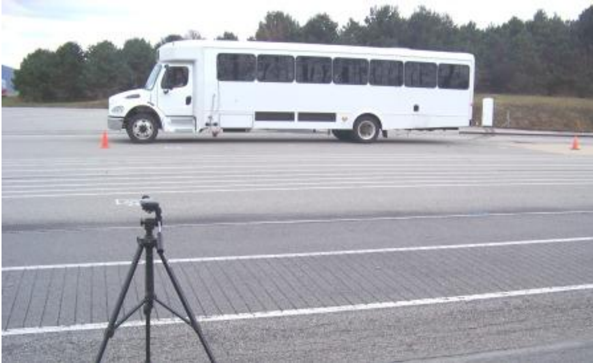
TEST BUS UNDERGOING EXTERIOR NOISE TEST
