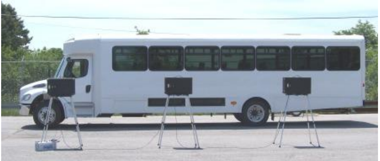
TEST BUS SET-UP FOR 80 dB(A) INTERIOR NOISE TEST
