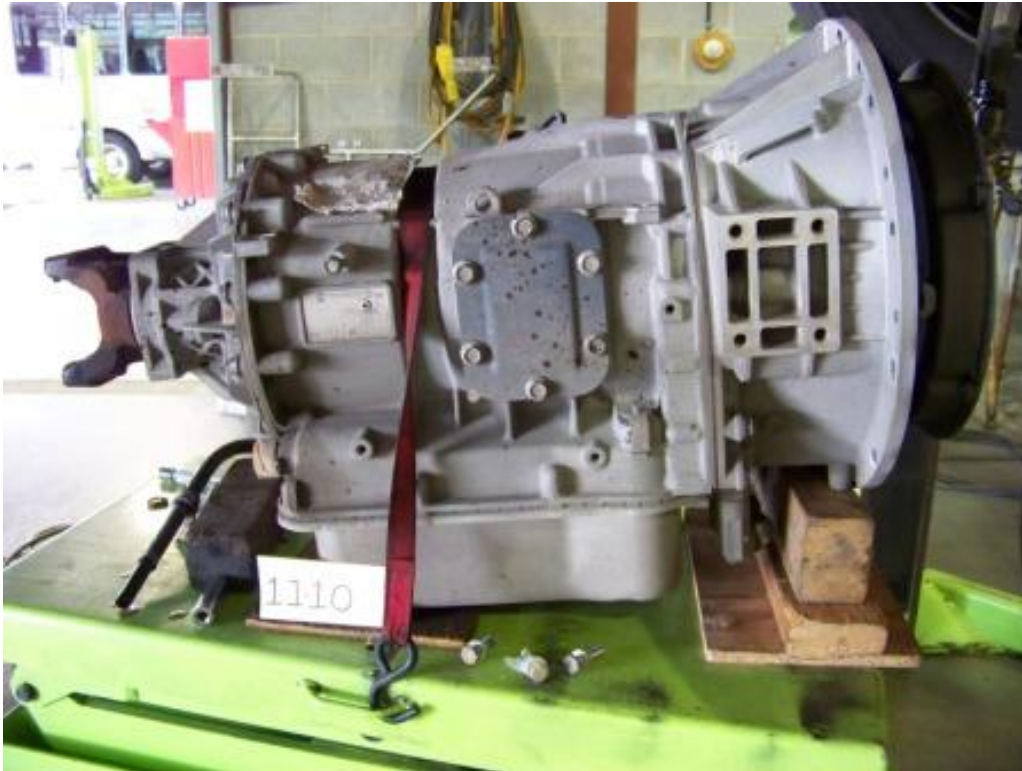
TRANSMISSION REMOVAL AND REPLACEMENT (8.00 MAN HOURS)
