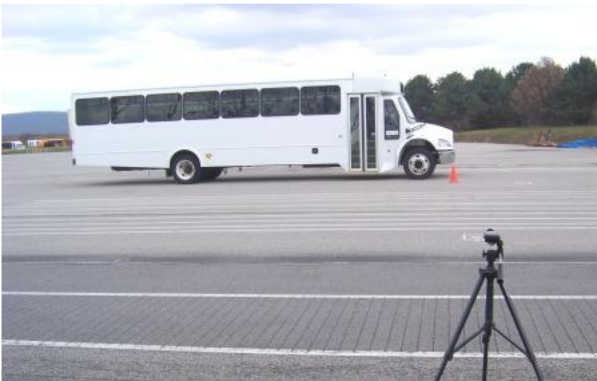
TEST BUS UNDERGOING EXTERIOR NOISE TEST
