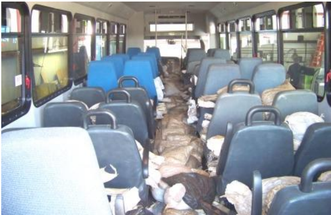
BUS LOADED TO 2.5 TIMES GVL (25,500 LBS)
