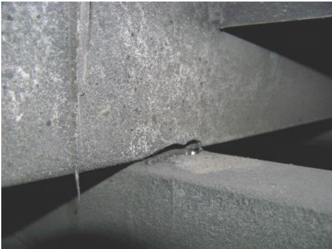
NUMEROUS BROKEN FLOOR CROSSMEMBER WELDS (8,207 TEST MILES)
