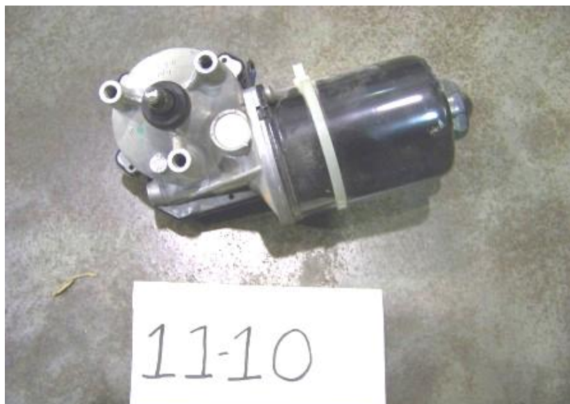
WIPER MOTOR REMOVAL AND REPLACEMENT (0.50 MAN HOURS)
