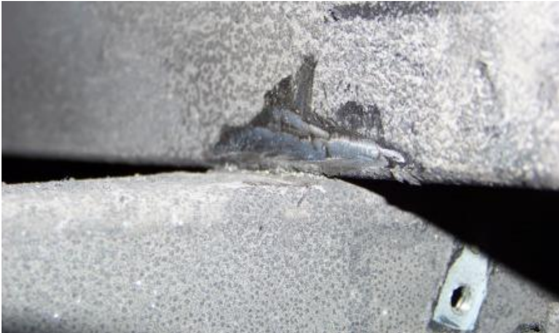
NUMEROUS BROKEN FLOOR CROSSMEMBER WELDS (8,207 TEST MILES)
