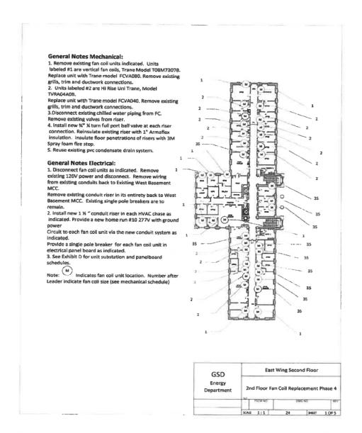
The above drawing illustrates the scope of the Energy Department fan coil replacement. The existing fan coil units were installed in the late 60's or early 70's and are failing at an alarming rate. This project provides new equipment with reheat for humidity control as well as UV light system to control airborne contaminates. The drawing illustrates the replacement of units in the House, but the total project involves Constitutional Offices and all three branches of government.
