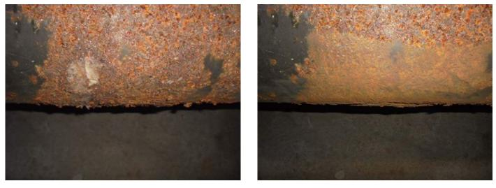
In terms of statistics, our investigation of 31 examples of chill water pipe identified a low and normal average corrosion rate of 0.5 mils per year (MPY), which we would consider very favorable. Testing in areas of the pipe having a smooth surface absent of any surface rust typically identified very high wall thickness at or just slightly below new pipe specifications to define very low internal corrosion activity.
