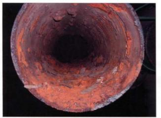
Figure 1. Heavy corrosion deposits along the length of a pipe. Severe pitting was found under the deposits.
