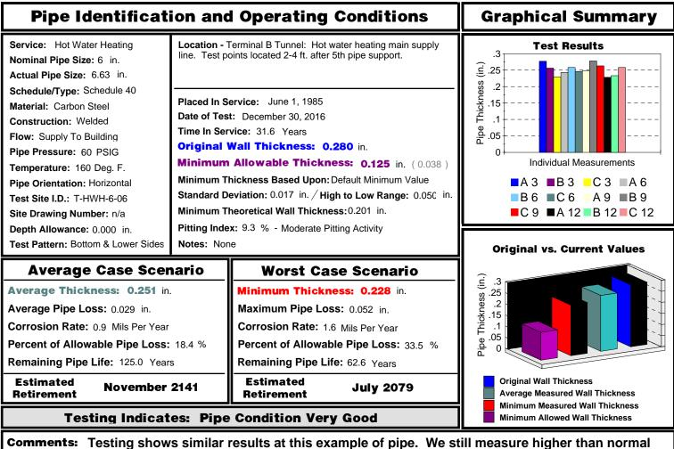
Comments: Testing shows similar results at this example of pipe. We still measure higher than normal internal pitting activity for a closed hot water system. Very long service life remains.
