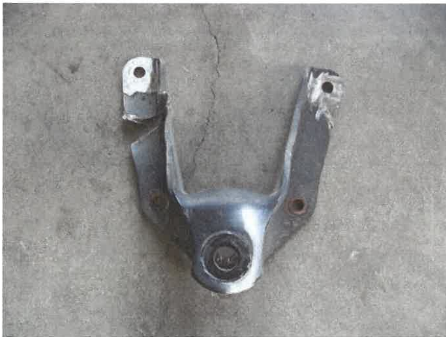
BROKEN RIGHT REAR SPRING HANGER (3,071 TEST MILES)
