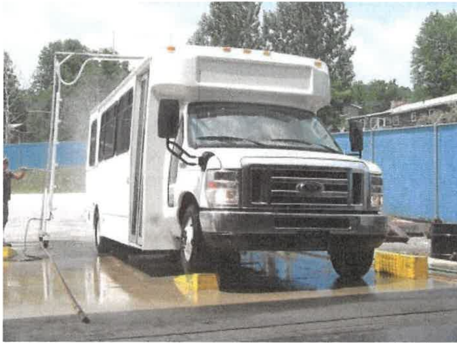
RIGHT FRONT WHEEL SIX INCHES HIGHER
