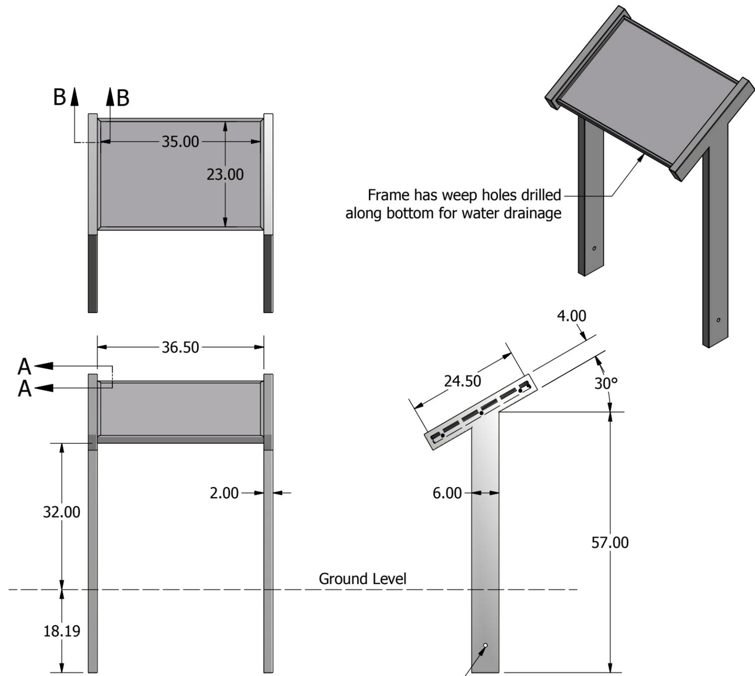
Holes for optional concrete reinforcement using steel rebar inserts
