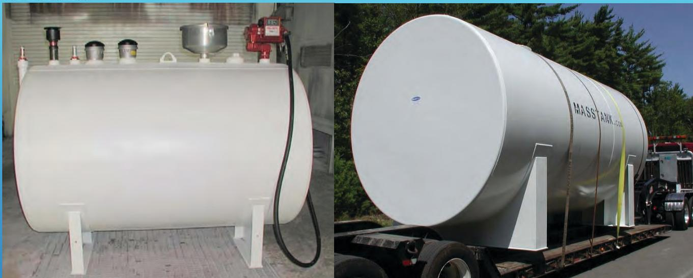
**Fireguard®** - Is a fire and ballistic resistant tank design that is patented and warranted by the Steel Tank Institute for 30 years. The design is 2-hour fire rated per UL-2085. All steel construction double wall tank features an inner steel tank with a unique lightweight thermal insulation material. An exterior steel wall provides superior weatherability and low cost maintenance.
