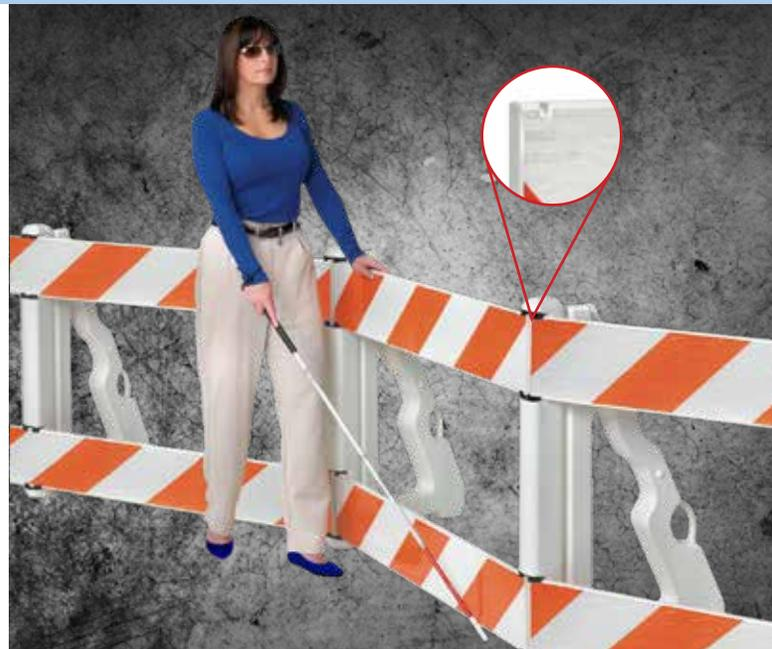
SafetyRail is designed for use with PSS Wave® Guide Rail. Upper Rail is smooth, continuous, and safer for the hand. Lower Wave Guiderail measures 1.5" from the ground which reduces potential for trapped cane tips. Wave "Notch" design (see insert) keeps guide rails securely in bushings.
