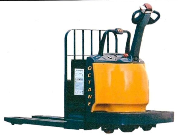
2021 OCTANE EP30A – This equipment is manufactured in the United States of America MODEL 30A – 6,000 lbs Capacity @ 24in Load Center 24V/280Ah Battery, Battery and Charger included, 48" Fork Length, 27" Across Forks, Polyurethane Tires, 12month/2,000hour Manufacturer's Warranty, Operator
