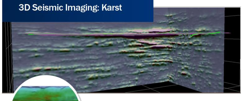
Our proprietary highresolution 3D seismic imaging provides unparalleled imaging of subsurface conditions which means more accurate site characterizations. better understanding of risk, more accurate construction estimates, and preconstruction subsurface remediation in karst terrains
