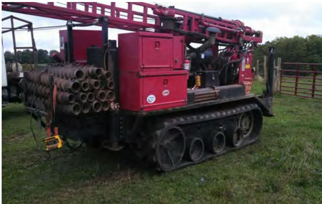
Diedrich D-50 Rubber Track Mounted Drill Rig
