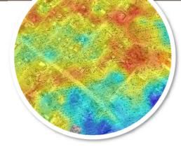
Our proprietary highresolution microgravity imaging provides unparalleled imaging of subsurface conditions, which means more accurate site characterizations, better understanding of risk, more precise remediation targets, and more accurate estimates of remediation costs.
