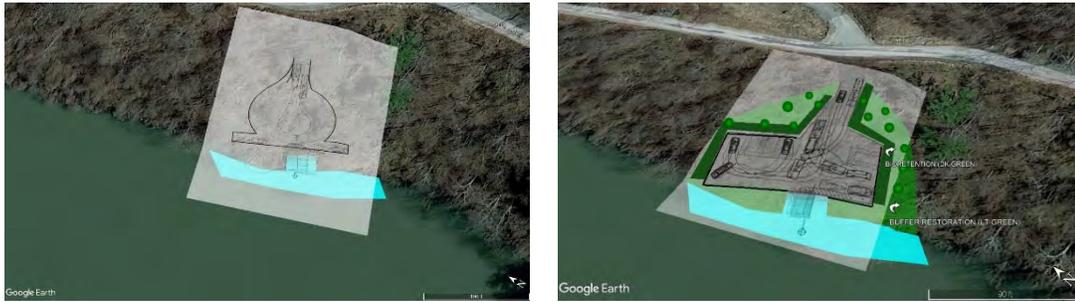
These sketches represent early concepts for vehicle access from the adjacent state highway to the docking, vehicle unloading, and parking facilities. These early preliminary concept studies have also included cost estimating for budgetary purposes. The cost estimates provide budgetary information for the Greene County Planning, and it also provides cost information to provide to funding agencies. The Pennsylvania Fish and Boat Commission is providing funding for the Wisecarver project.
