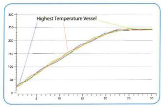
Patented DuoTemp Control automatically measures the temperature in each vessel and dynamically controls the run based on the most reactive vessel.
