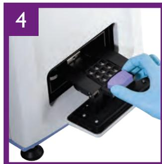
4 Biochip carrier loaded into Evidence Investigator
