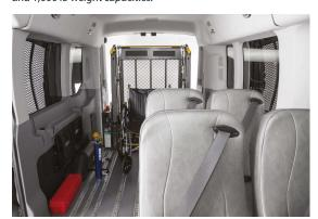
Inside view of paratransit van with SmartFloor system and wheelchair lift in rear location.
