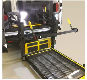
Side and rear access wheelchair lifts are available with 800 lb and 1,000 lb weight capacities.
