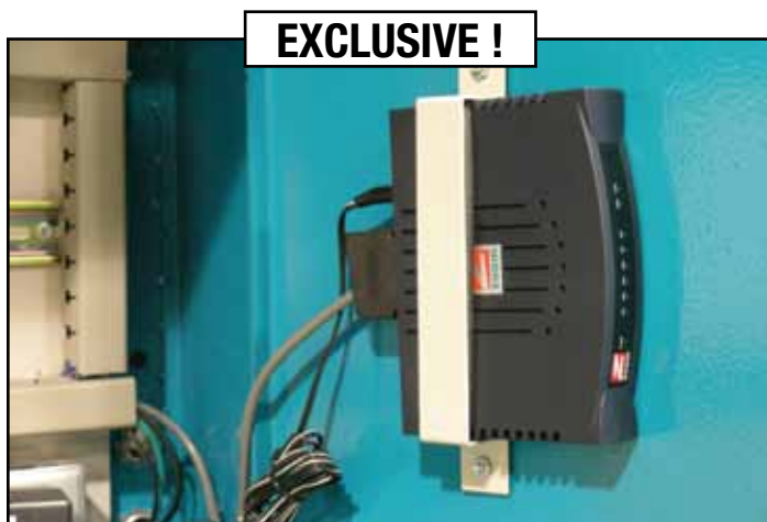
Remote Diagnostics System: Onboard microprocessor connects via phone modem for instant worldwide service. Direct link to A.W.T.'s central diagnostics computer provides quick identification and correction of malfunction sources. Onsite service calls are eliminated in most cases.
