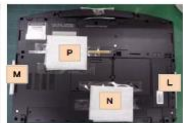
L. CN Cover M. User Upgrade Pocket Cover N. Bottom Cover P. Config Area Cover
