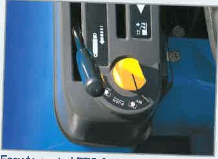
Easy to control PTO Switch Turn the rear or mid PTO on or off with the simple and easy turn of a switch
