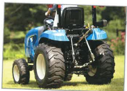
High efficient 3-point hitch Improves your working speed and safety with quick reponse and maximized lift capacity of 3-point hitch
