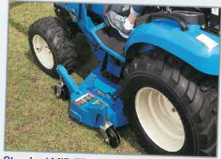
Standard MID PTO 2000 RPM Mid PTO for optional height adjustable 60" mid-mount mower that provides a smooth and beautiful cut
