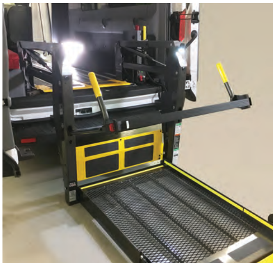
Side and rear access wheelchair lifts are available with 800 lb and 1,000 lb weight capacities.
