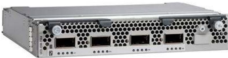
The Cisco UCS 2304 connects the I/O fabric between the Cisco UCS 6300 Series Fabric Interconnects and the Cisco UCS 5100 Series Blade Server Chassis, enabling a lossless and deterministic Fibre Channel over Ethernet (FCoE) fabric to connect all blades and chassis together.
