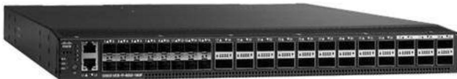
The Fabric Interconnect provides high-speed upstream connectivity to the network, or converged traffic to servers through its 40 Gbps ports, but also allows for Fibre Channel connectivity to SAN switches like the MDS, or alternately directly attached Fibre Channel to storage arrays.
