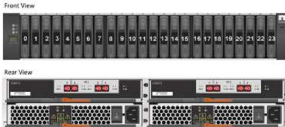
Combined with the 3 disk shelves and 72 1TB Solid State disks (SSD), this solution can provide over ample horsepower and over 60TB of raw capacity, all while taking up minimum valuable rack space. This makes it an ideal controller for a shared workload converged infrastructure. For situations where more performance is needed, the A700s would be an ideal fit. ONTAP 9.3 is used with the AFF A700s storage platform in our design.
