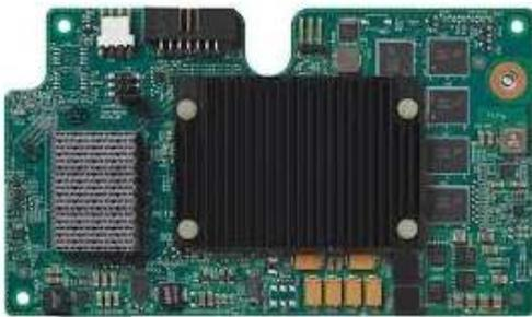
Cisco UCS 1340 VIC delivers 80 Gbps throughput to the Server and helps reduce TCO by consolidating the overall number of NICs, HBAs, cables, and switches; LAN and SAN traffic runs over the same mezzanine card and fabric.
