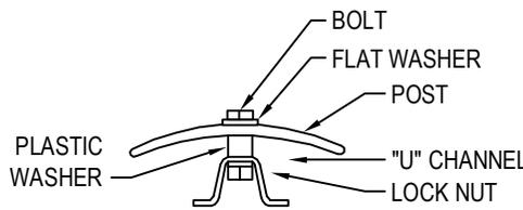
FG 96 STEEL ANCHOR ATTACHED TO POST
