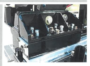
Utilizing the largest adjustable slide track bushing in its class, the EZIV extension maintains integrity of the slide track function for reduced lifecycle costs and superior performance.
