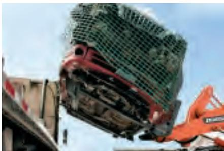
Easily lift, carry and place materials. Available with with 48" or 60" tines for DL200-5, DL200TC-5, DL220-5, DL250-5 and DL250TC-5 wheel loaders.
