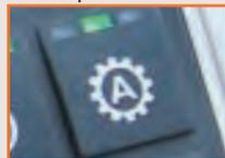
**Auto 2-4 with Manual Kickdown** gives you automatic shifting between gears 2 through 4, with a manual downshift into first gear when you need it. It provides the best performance for less demanding work conditions.
