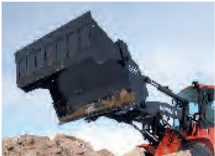
Leveling, dozing, digging, grappling, loading and dumping – this multi-purpose bucket is ready for whatever you've got. Capacities range from 3.5 to 4 yd<sup>3</sup>.
